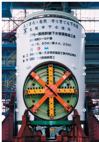
▲ Construction of the Bandai ~ Hannan trunk sewer (Vertical-to-horizontal shield machine) Shield diameters Vertical diameter : 5.90 m Horizontal diameter: 4.20 m Type: Slurry shield (Vertical) Earth pressure balanced shield (Horizontal)
