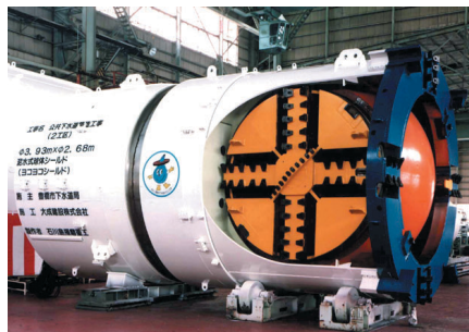
▲ Construction of the Shimoji sewer (Horizontal-to-horizontal shield machine) Shield diameters Main shield diameter: 3.93 m Sub-shield diameter : 2.68 m Type: Slurry shield
